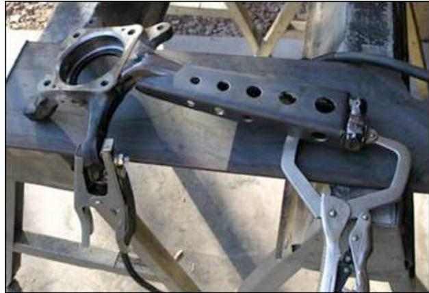
Tack the gusset to the spindle (left photo) Pictured on the right below is the finalized weld
