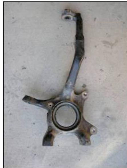
Finish disassembly and remove the spindle from the vehicle. Here is the knuckle, taken down to where nothing else is attached other than the grease seal that the axle rides in
