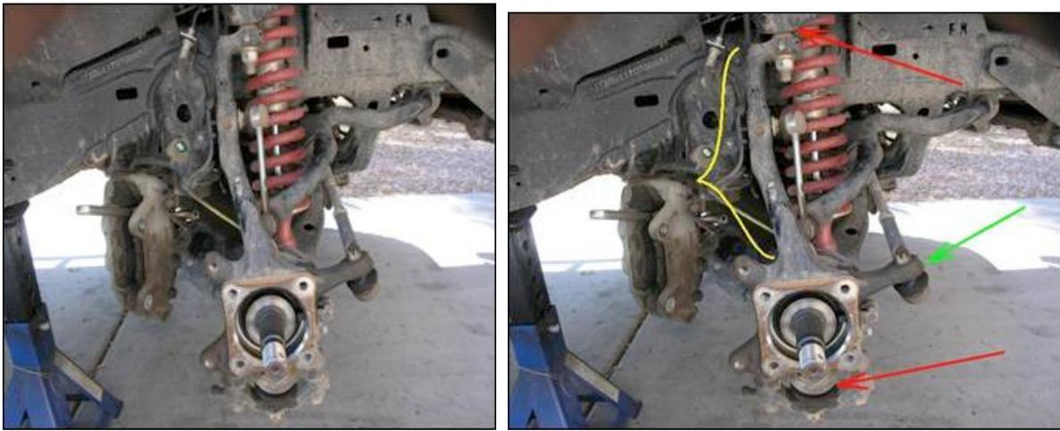
When disconnecting the sway bar link, inspect them for damage such as bending as pictured at the arrow below, or leakage from the boots. If you find damage, now would be a great time to upgrade to the All Pro heavy duty sway bar links and the sway bar centering collars we offer to prevent the problem from happening again.
