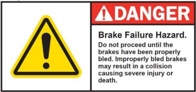
7. Before test driving your vehicle, make a final check of all brake lines to ensure all connections are tight and do not leak. The brake pedal should be firm at this stage. After the first 100 miles recheck all the lines and connections for tightness and leaks.
