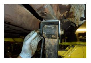
Install the passenger side spring the same way as the driver side.
