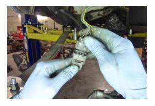
Plug in the E-Locker wires (or air hoses) if your vehicle has this feature.
