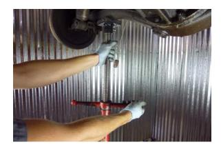
Remove the lower end of the shock using a large screwdriver or pry bar and set the shock aside.
