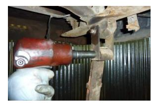
Remove the lower rear shackle bolt nut using a 19 mm socket.
