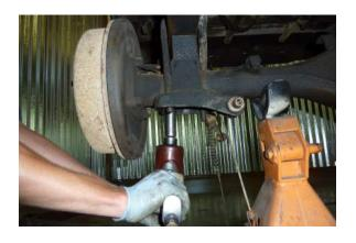
Repeat the above steps on the passenger side U-bolts, pad, pad retainer and U-bolt plate.
