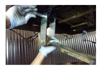
Install the shackle mount bolt and nut on the passenger side. It is okay to snug this nut but do not tighten all the way yet.
