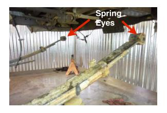
Raise or lower the vehicle so that the rear eyes of the leaf springs are about 6 inches away from the frame.
