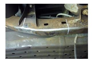
Using a grinder, remove any rust or undercoating where the front mount is to be positioned to provide a good clean surface for welding.
