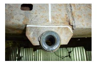
Beginning on the driver side, mark the outside of the rear shackle mount and cut it off with the cut-off wheel.
