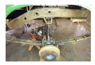
Stack 6" worth of wood between the frame and the rear of the leaf springs. Four 2X4's worked just right. (2X4's are actually 1.5" thick) It may be necessary to raise the vehicle a bit to accomplish this step. Once the wood is in place on both sides, lower the vehicle until the full weight of the rear of the vehicle is resting on the rear axle assembly and leaf springs.
