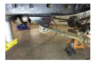
While lowering the vehicle guide the front of the leaf springs into front mounts.
