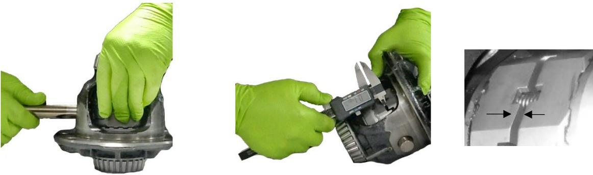
11.) **Reinstall the Cross Pin and Roll Pin** Use a punch to reinstall the roll pin
