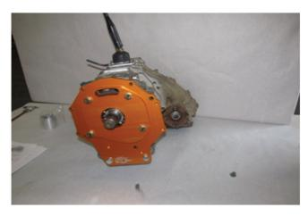
**STEP 12**Install provided coupler to transmission
