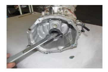
**STEP 13**Install seal housing and seal with a rubber mallet.
