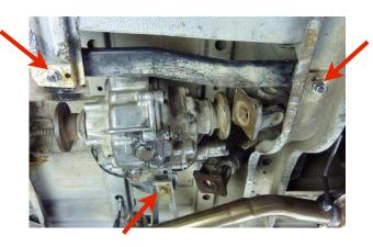
Remove the (3) transfer case mount nuts using a 14 mm socket.
