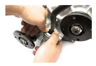
Align the grooves in the shifter guide with the pins that are inside the shifter cavity.
