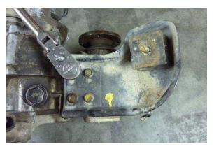
If the fluid has been drained, turn the transfer case over and remove the passenger side bracket by removing the (4) bolts using a 12 mm socket. This bracket will not be used with the new cradle kit.
