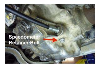
Disconnect the speedometer cable by removing the bolt using a 10 mm socket. Once the bolt is removed pull the cable out.
