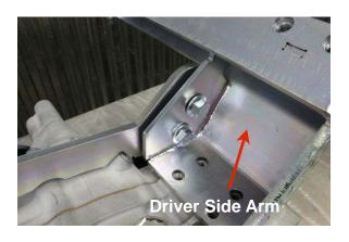
Position the driver side arm as shown and install the two large flange bolts as shown.
