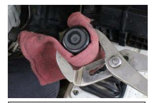
Picture showing hard-to-remove shift knob removal.
