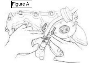
Illustration showing shift lever guide removal procedure.
