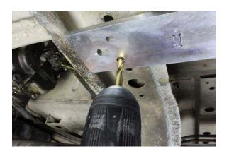
Again, using the hole in drivers side arm as a guide, drill a second hole in the cross member using the 1/4" drill bit supplied in this kit.
