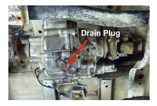
Position a pan under the drain plug. Remove the drain plug using a 24 mm box end wrench (or a 3/8" extension if you have the internal square plug). This is a good time to change the transfer case fluid if it needs changing. In addition, draining the fluid will make the job a lot cleaner. However, draining the fluid is not required. This job can be done without draining the fluid if you are very careful.
