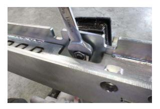
Install the lock washer and nut on mount #3 and tighten. (18.5 to 25 ft. lbs.)
