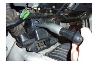
Step 6 Insert the vacuum hose in the hole and turn on the vacuum cleaner.
