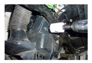
Drill the centering hole with the drill bit of
