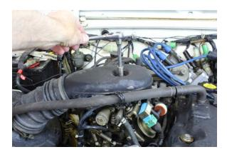
Remove the air intake case nut using a 10mm socket.
