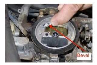
**Step 10** Position the nozzle with the bevel "up" as shown.
