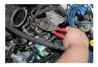
**Step 8** Remove the air intake case mounting stud for easier vent tube installation.
