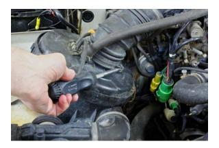
**Step 3** Loosen the air intake duct clamp.
