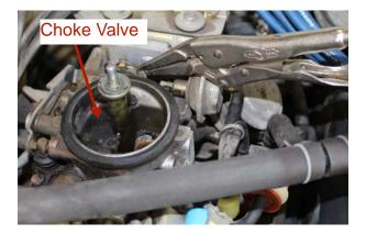
Insure that the choke valve is closed. If it is open, block it closed using locking needle nose pliers as shown. This will reduce the risk of accidentally dropping the nozzle down the throat of the carburetor.
