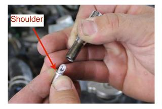
Select the correct socket. The socket should be large enough to barely fit over the nozzle yet small enough to fully contacting the shoulder. We found a 7/32" 6 point deep socket worked well.
