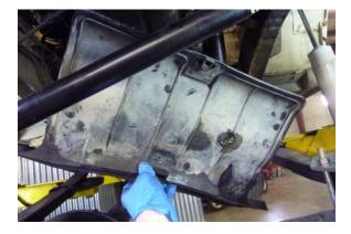
Remove the splash panel by lifting up, sliding rearward and down. Then set the panel aside.
