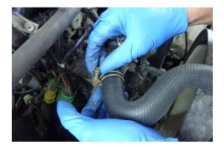
Slide the hose clamp into position at the thermostat housing end.
