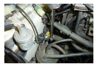
Tech Tip 33 B This shows proper worm gear hose clamp removal.
