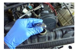
Step 38 If installed, remove the radiator cap.
