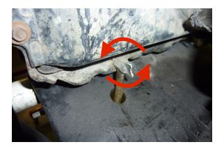
Step 3 Open the drain valve by tuning it counter clockwise.
