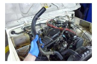
Install the lower hose assembly in reverse order of removal.
