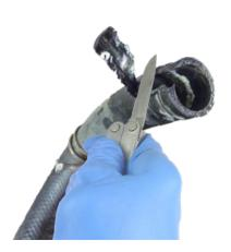
In some cases it may be necessary to cut the hose with a sharp pocket knife as shown here.
