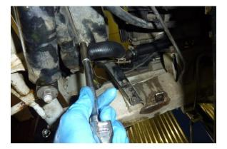
Step 31 Position and secure the (2) clamps, one at the radiator and one the inlet pipe.
