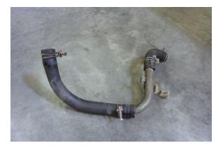
Once the lower radiator hose assembly has been removed, loosen the other 2 hose clamps.
