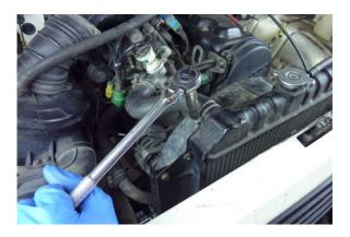
Step 6 Loosen the hose clamp using a 10 mm socket.
