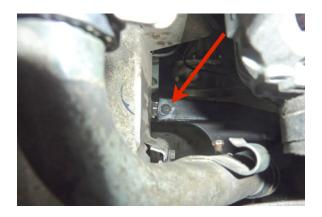
Step 24 Remove the passenger side screw in the same way.
