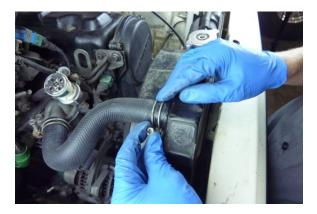
Slide the hose clamp into position at the radiator end.
