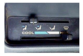
Place the heater temperature control in the "HOT" position.
