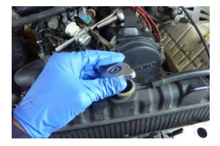
Remove the radiator cap to allow the coolant to drain faster. Inspect the cap and replace if needed.
