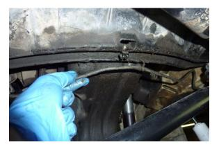
Step 22 Unclip the brake line as shown.
