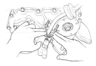
Illustration showing lever guide removal procedure.
