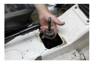
Slide the lower shifter boot off the top of the shifter handle.
