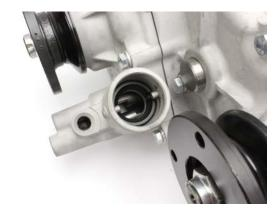
Bushing shown correctly positioned.
