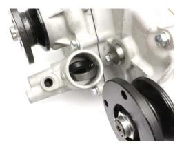
Continue rotating the bushing, using the pins as pivot points, until the bushing drops into place.
