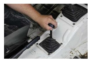
Place the transfer case shifter in NEUTRAL .Then remove the shift knob by twisting it in a counter-clockwise direction.
