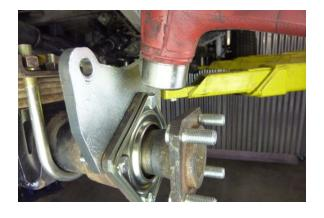
Step 57 Bend down the (4) tabs on the SJ 410 Backing Plate by striking them with a ball peen hammer.
