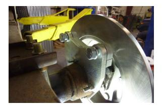
Step 63 Insert the (2) supplied M12X1.25X35mm bolts and lock washers as shown.
