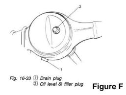
If Gear Oil was lost from the rear axle housing during this repair you will need to replenish it. Even if you did not loose any fluid, it is a good idea to check (& fill if needed) this level before putting this vehicle back into service.
