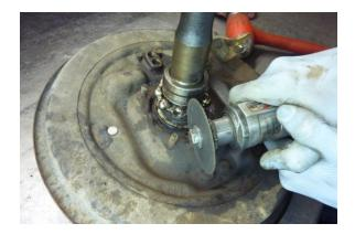
Step 28 Cut the bearing cage using the cut off wheel.
