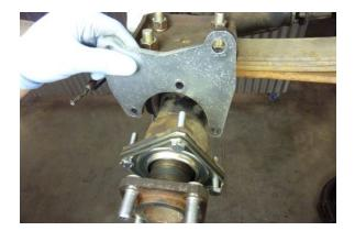
Install the supplied axle plate on the (3) M8X1.25X35mm bolts.
