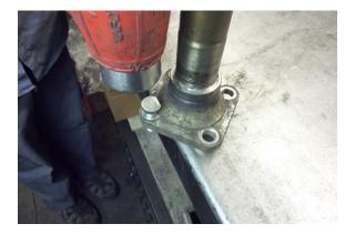
Strike the stud with a ball peen hammer until the head of the stud contacts the axle hub.
