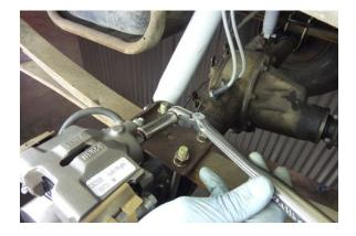
Thread the banjo bolt into the caliper. Torque the banjo bolt to 20 ft. lbs.
