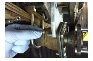
Step 55 Install the (4) supplied M8X1.25 serrated nuts on the (4) M8X1.25 bolts.
