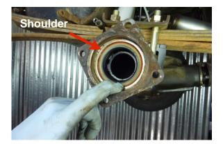
Stop driving the seal when it reaches the same location as the one just removed or about 1/16" inside the axle housing shoulder. (See next Tech Tip)
