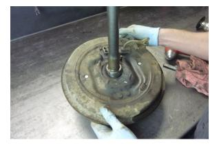
Step 31 Remove the brake backing plate.
