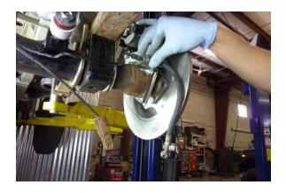
Step 68 Position the brake line as shown.
