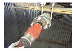
Continue installing the axle shaft until the bearing hits the axle housing. Once the bearing is started into the axle housing, strike the axle using the ball end of a ball peen hammer as shown.
