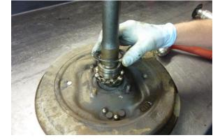
Step 26 Remove the two outer bearing race halves.
