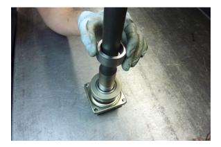
Step 44 Place the bearing collar on the axle as shown.
