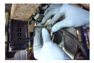
Step 69 Thread the solid brake line into the flexible line.
