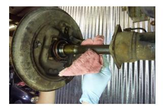
Step 14 Remove the axle, backing plate and bearing assembly and set it aside.
