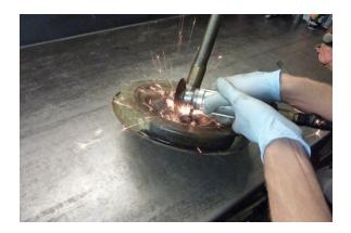
Step 24 Make a second cut through the outer bearing race.
