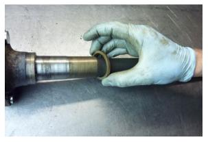
Step 35 Remove the bearing spacer.
