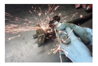
Cut the bearing collar (See Figure A to see the Collar) about 3/4 of the way through using the cut-off wheel.
