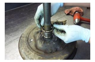
Step 30 Remove the lower bearing cover.
