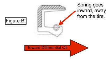
Tech Tip 17 The correct seal orientation.
