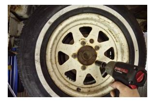
Tech Tip 13 (Continued) Leave the axle, drum and backing plate in the rear axle housing and remove the wheel assembly using a 19 mm socket.
