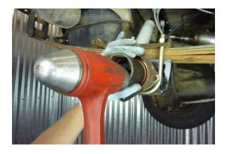
Step 19 Carefully and evenly drive the seal into the axle housing.
