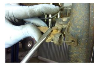
Remove the parking brake pin using a standard screwdriver. Lay the parking brake cable out of the way for now.
