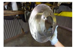
Install the supplied brake rotor onto the wheel studs.
