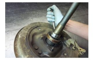
Step 23 Rotate the outer bearing race 180° (or 1/2 turn)
