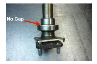
Step 46 Bearing collar properly positioned.
