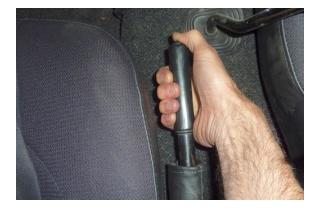
Release the parking brake if applied (Lever down).
