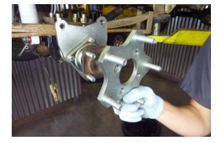
Step 58 Install the axle hub on the axle studs.
