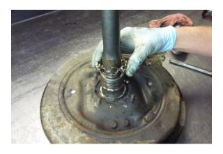
Step 29 Remove the cage and any ball bearings if there are any remaining in place.
