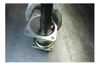
Install the supplied disc brake backing plate on the axle, on top of the SJ 410 backing plate, as shown.
