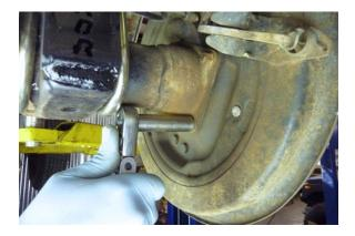
Remove the (4) backing plate nuts using a 14 mm socket.
