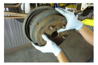
Remove the brake drum and set it aside.
