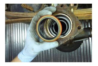
Correctly position the new seal in the housing. See next tech tip for correct
