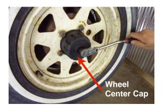
Remove the wheel center cap by removing the (1) center bolt using a 14 mm socket.
