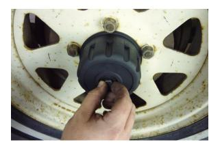
Install the wheel center cap and tighten the bolt.
