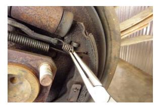
Step 17 Remove the rod spring.
