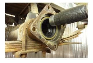
Start the seal by tapping gently with a small hammer.
