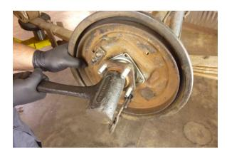
When the splines of the axle shaft align with splines inside the differential (See Figure J) you will be able to push the axle shaft farther inward.
