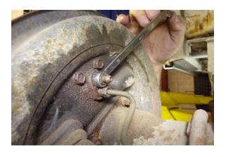
Place a pan under the brake bleeder screw and remove the brake bleeder screw using a 10 mm box end wrench.
