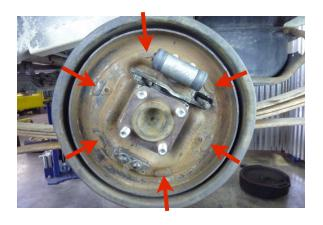
Lube the backing plate bosses with a good quality brake parts lubricant in the (6) locations shown above.
