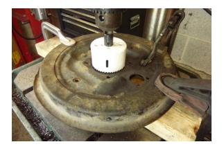
Turn the drill press on and slowly feed the hole saw into the backing plate.
