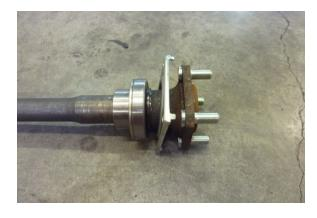
Install the axle bearing retainer using the pipe and hammer just as you did the axle bearing.
