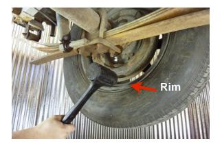
Pound on the inside of the rim (or tire) with a large dead blow hammer until the axle, brakes and wheel assembly comes out of the axle housing.
