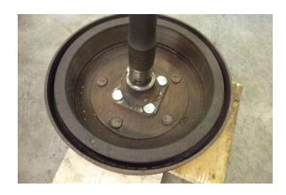
Align the axle hub stud holes with the brake drum holes and insert a new hub stud. Make sure the flat on the hub stud faces the center of the axle. Drive the hub stud into place with a hammer. Repeat the process on the remaining (3) studs.
