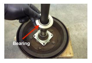
Install the bearing on the axle shaft with the flat side up.
