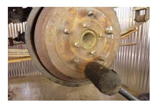
Install the brake drum and pound the axle and bearing farther into position with a dead blow hammer as shown.
