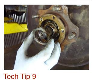
Now would be a good time to service (remove, clean, repack and adjust) the wheel bearings.
