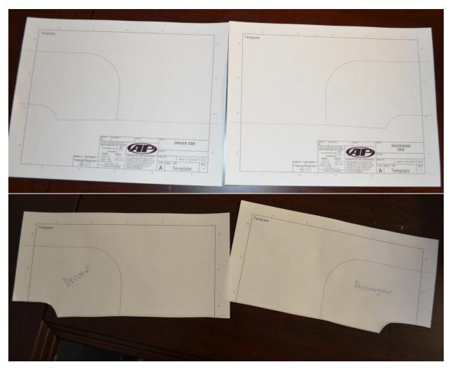
After template has been cut out, locate the raised edge on the bumper around the stock fog lights. This edge is the reference to use to position the template.
