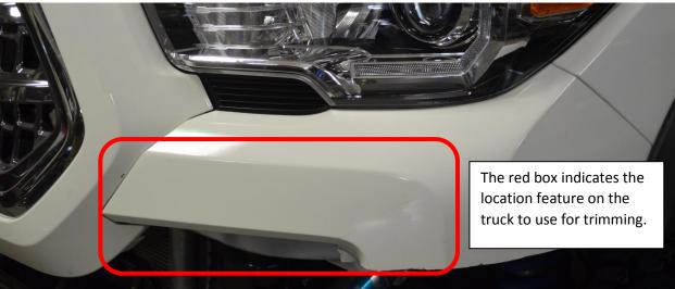
Using painters tape, tape the template to the bumper being careful to match the lines on the template with the lines on the bumper.
