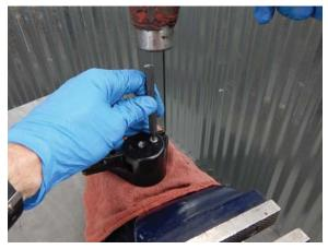
Tech Tip 12 A It may be necessary to recess the pin using a hammer and punch.
