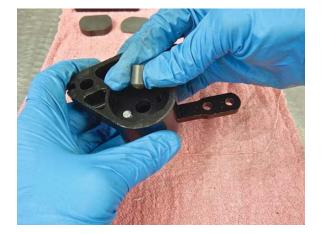
Step 15 Install the actuating pin with the rounded part downward.
