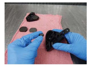
Step 5 Remove the actuator pin.
