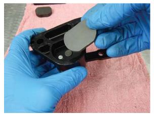
Step 16 Install the pad plate.
