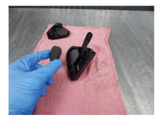
Step 3 Remove the pad from caliper housing #1.
