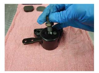
Step 13 Reinstall the adjustment bolt and lock nut.
