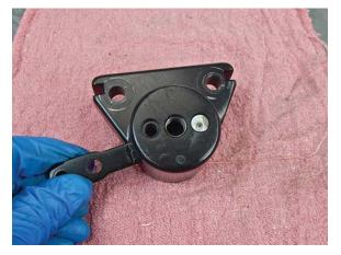
Tech Tip 12 B This shows the lever and pin properly installed.
