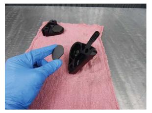
Step 4 Remove the pad plate.
