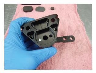
Step 14 Turn caliper housing #1 over.
