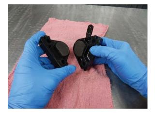
Step 2 Separate the two housings.
