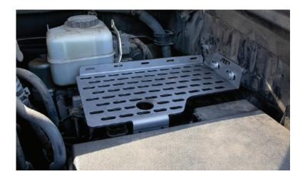
**1.** Open the hood and locate the space above the fuse box on the driver side of the engine bay.
