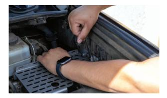
**6.** Once the bracket is in the desired position first tighten the bottom bolt then the two side bolts.
