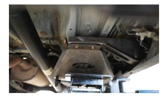
11. If you have not already done so, push the front mounting bracket against the inside of the driver frame rail. The mounting bracket should be approximately centered between the upper and lower edges of the frame rail. Adjust the skid plate if needed so it is covering the bottom of the gas tank. It may be necessary to clearance the upper or lower edges of your frame rail if there is interference between the frame rail and the mounting bracket.
