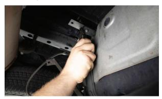
**8.** Attach the secondary mounting bracket to the top of the passenger mounting bracket using the supplied hardware as shown. Tighten this bolt.
