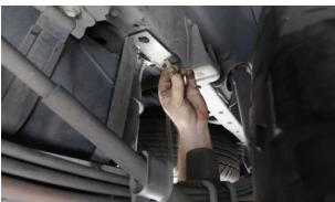
**6.** Using the supplied hardware, attach the secondary mounting bracket to the factory cross member as shown. About half of the bracket should be supported by the factory cross member and the other half should hang off. Align the bracket so it is in line with the cross member and tighten the mounting bolt.
