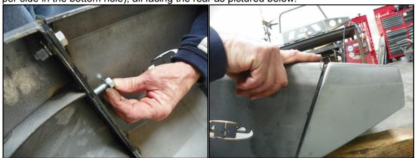
Align flush with the outside of the bumper, and tighten down snug. You do not need to attach the braces yet.
