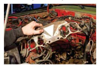
Now that you have removed your stock header, it's time to install your new Rock Ripper™ Header. Note: We recommend installing new hardware with your header and using anti-seize.
