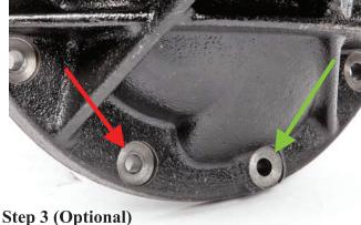
If you are using a Rock Assault housing, you will need to use the studs that came with the Rock Assault housing for the two lower studs.
