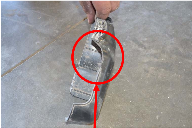
Cut out on top of plastic cover must be trimmed opened more on right side.
