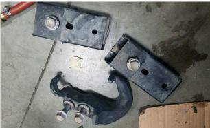
**12.)** Using the supplied relocation tabs, relocate the two brackets connected to the power steering cooler line back towards the radiator. Once the brackets have been relocated, it may be necessary to bend the brackets upwards a little to clear the bolt head and prevent the steering cooler line from rubbing on anything.
