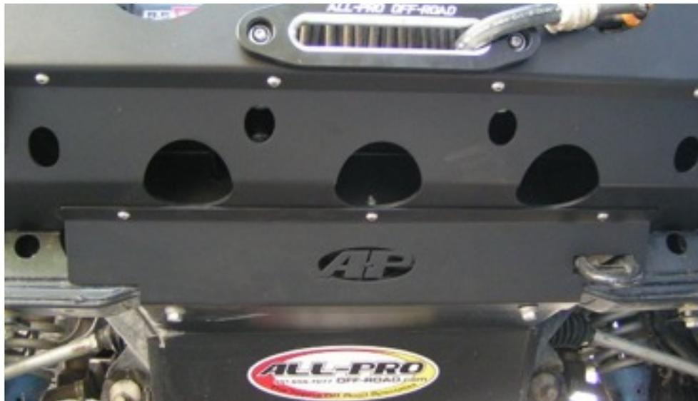
16. Measure and mark 1 inch below flush on the fender well plastic. Trim along your 1" mark as pictured. Once the fender well is trimmed it can be tucked under the bumper
