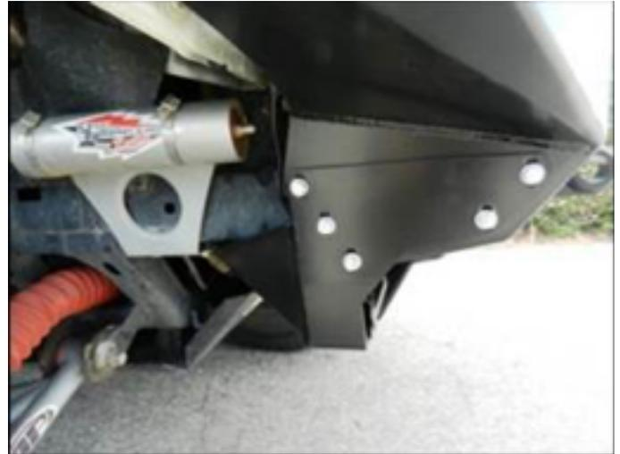
15. Now you can install the valance (E) onto the lower center section using 3 Button Head Bolts 5/16 x 1"L, each with a flat washer, a lock washer and nut. Use the two factory skid plate bolts to attach the bottom, as pictured.
