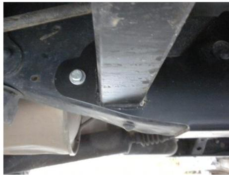
You will use the remainder of the Hex Head bolts to hold the plate of the slider to the frame in already pre-drilled holes in the frame
