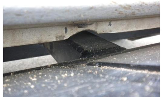
Next, drill 4 holes in the frame using a 5/16" drill bit for the front leg and insert the Self Tapping Screws (Lower Left). Then drill a 3/8" hole in the rear and insert a Hex Head bolt with flat washers and locknut. (Lower Right).
