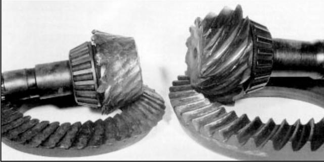
You just installed a new ring & pinion set and you're ready to feel the power. Hold on, don't burn rubber yet. That new gear set may become scrap metal faster than you can say "burned gear syndrome".
