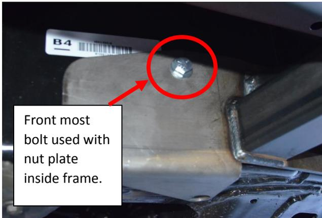
Front most bolt used with nut plate inside frame.
