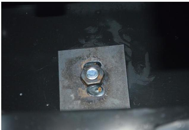
Nut plate on backside of frame covering rectangular hole.
