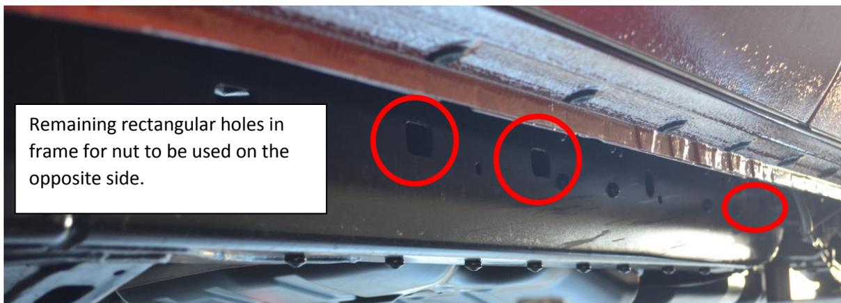
Remaining rectangular holes in frame for nut to be used on the opposite side.
