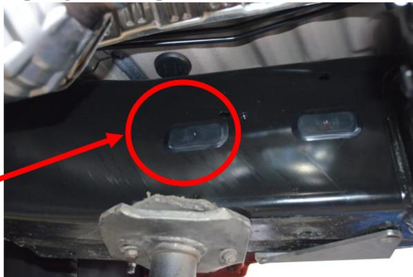
Removable plastic cover allowing easier access to align nut plate on the backside of the frame.
